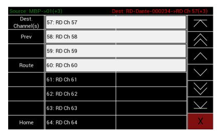
The screen will then change to the Source Channel(s) screen Select the channel(s) that need to be routed and then press Next to go to the Destination Channel(s) screen
