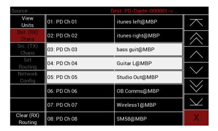
It is also possible to remove individual and multiple routes in the RX channels screen. Simply select the channel(s) that need to be unrouted. The background of selected channel(s) will turn white
