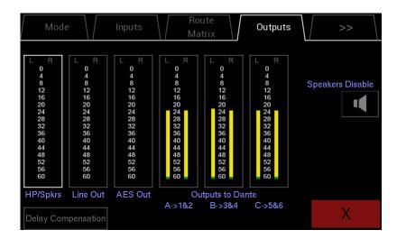
This page is split into seven areas, 6 stereo meters and a control area. Select an output by touching its meter. Controls for that output will then be displayed in the control area
