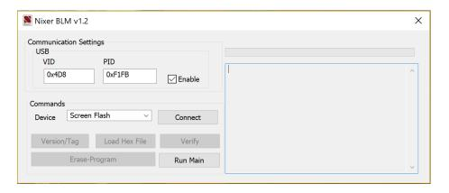
Once the program is running change "Screen Flash" to "Main CPU" via the dropdown menu and click connect
