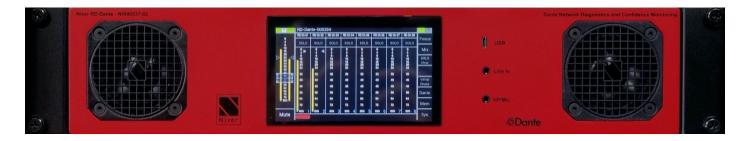
The front of the unit has a large 5" (127mm) Capacitive touchscreen TFT display plus two full range 63.5mm diameter speakers in optimally tuned and ported enclosures for confidence monitoring. The front panel is the location for the 3.5mm jack headphone output with mic input, the 3.5mm stereo line input jack and the USB micro AB connector for installing firmware updates.
