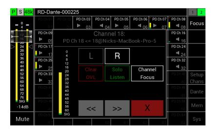
On pressing a Channel Cell the Channel Assignment window will open overlaying the Main Input Screen
