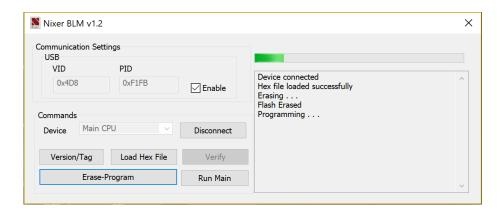
When the device has been programmed the status window will say "Programming completed. Click Run Main and your unit will reboot with its updated software
