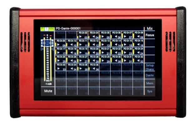
The front of the unit has a large 5" (127mm) Capacitive touchscreen TFT display plus two small speakers for confidence monitoring.
