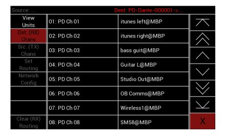
Example of viewing the RX channels of the selected device
