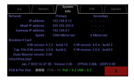
Network connection parameters and firmware versions are displayed on this page
