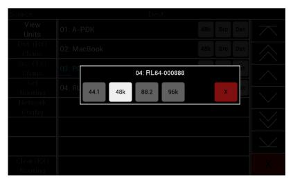
On pressing the sample rate of a device in the device list the screen above will be displayed
