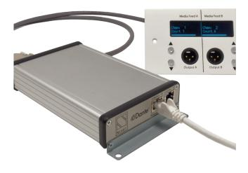
The remote controller allows the independent selection for each output from the incoming Dante stream. Each output displays the selected Dante channel name and output signal level on the OLED display. Channel selection is made via scrolling up/down the available Dante channels via a pair of switches for each output
